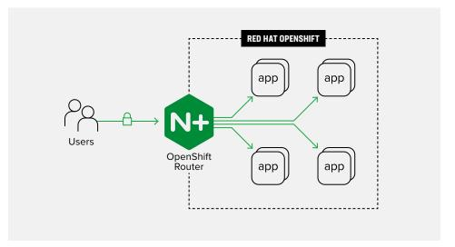
Use the NGINX Plus OpenShift Router for SSL termination, routing, and load balancing.
