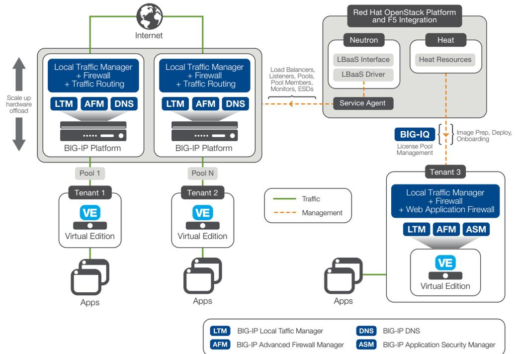
Figure 1: F5 OpenStack deployment test architecture
