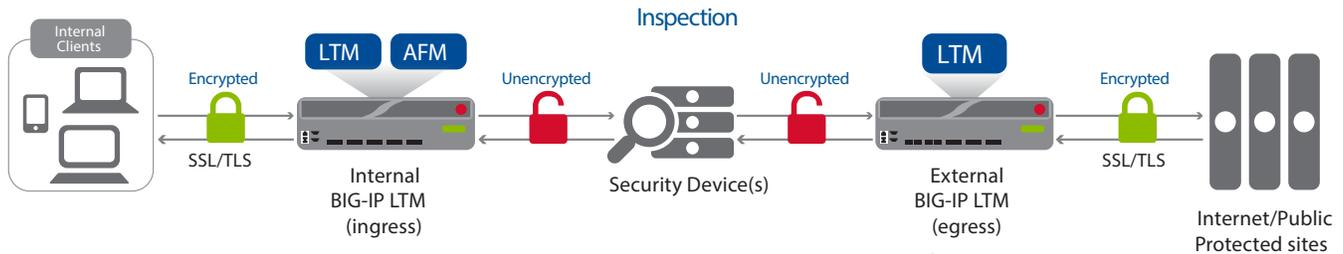
**Figure 1:** Logical configuration diagram of the SSL intercept configuration using an ingress and egress BIG-IP system
